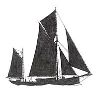
**Ketch** A two masted sailing vessel where the mizzen mast is ahead of the rudder. The rig is similar to a schooner but the main mast (the tallest mast) is the first mast, not the second mast. Ketches were common in 19th century Europe but rare in Nova Scotia until they became very popular for yachts in the 20th century.
