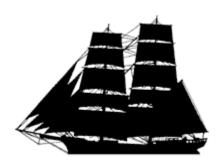
**Brig**, a two masted vessel square rigged on both masts. The brig is a very old and efficient sailing rig, and the class was still in use up to the very end of commercial sailing ships. Only a few brigs were built in Nova Scotia yards, but they were very common in European waters.
