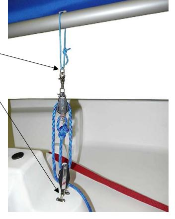
10. <u>Attach sprit.</u> Put one end of sprit into loop at peak (top corner) of sail. Push the sprit up and out until you can hook the other end into the small bowline of sprit adjuster. Pull sprit adjuster line below cleat to tighten. Tighten just until diagonal wrinkles disappear from sail, then cleat line.
