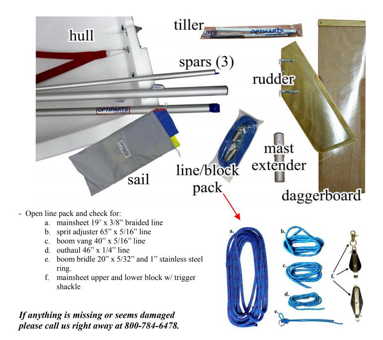
2. <u>Install mast extender.</u> Your spars were constructed for alternate use in the Optimist Dinghy, which has a deeper cockpit than the OPPI. The mast extender raises the sail and boom allowing an additional 4" of headroom (and that's a good thing!). Remove the end plug in the top of the mast (the largest spar), by tapping it out with a screwdriver.
