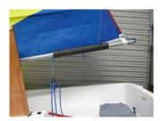
To cushion boom-to-head contact for beginners, tape or plastic wire tie a 24" piece of pipe insulation just aft of boom bridle.
