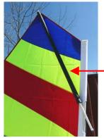
Slide a section of pool noodle or Pipe insulation over the upper end of the sprit to help prevent turning turtle in event of capsize.
